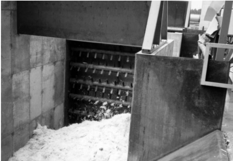
The combination of a slow moving live bottom apron, triple beaters and a leveling drag assures a smooth, even discharge of feathers.
