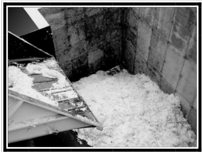
The notched side of the ALLOY Bin is custom designed for Truck Dump loading of the Bin. Ease and flexibility of filling permits the ALLOY bin to be mounted partially above ground, simplifying discharge conveyance, maintenance and clean up.
