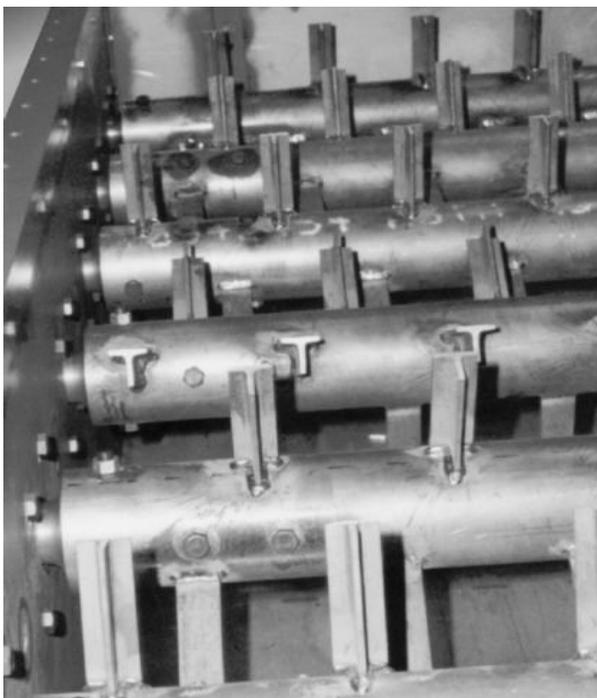
Heavy duty construction, as seen in this picture of the ALLOY picker assemblies, coupled with extensive use of stainless steel and other non-corroding and corrosion resistant materials, help the ALLOY Raw Feather Bin provide years of service without maintenance concern.
