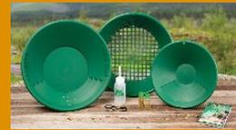
The most basic piece of prospecting equipment is the gold pan. Size, color, and shape are really a matter of personal preference. It's good to have a variety of different sizes of gold pans on hand, so check out [gold pan options and kits here.](#)
