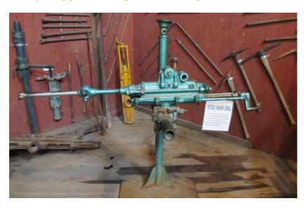
Perhaps the most important improvement made to mining technology over the years has been to drilling and blasting. In the early days, black powder was the only blasting agent available. To use it, holes had to be pounded into rock by hand. Working in teams of two, one miner would hold a pointed steel chisel while the other hit it with a sledge hammer. Each hole had to be hand drilled to six or eight inches in depth. What slow, tedious, and tiring work!
