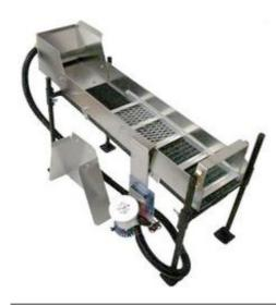
Process more material and get more gold! Time to step up your gold mining efforts? Check out power sluice kits and highbankers here. A power sluice or highbanker is basically a sluice box with height and mobility and a pump. It is mounted on a 4-legged stand that gives the sluice box the correct slope. Instead of positioning in the creek like a hand sluice, pump the water up from the stream into the sluice or highbanker. Made in the USA!
