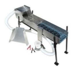
A power sluice or highbanker is basically a sluice box with height and mobility and is motorized. It is mounted on a 4-legged stand that gives the sluice box the correct slope. Instead of being put right in the creek like a hand sluice, an engine with a water pump and some hoses gets the water up from the stream into the sluice or highbanker. Gold-bearing gravel and dirt is shoveled into the hopper of the power sluice / high
