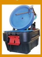
If you don't have the muscle power or time, let a spiral panning machine help you separate the gold from your concentrates and black sand much more quickly and easily! The Desert Fox Automatic Gold Panning Machine is designed to conserve water and will operate on just three gallons. It sets up quickly
