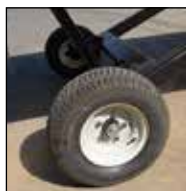
PNEUMATIC TIRES OPTION Service Range will be 40" to 66" model AY-PNTR
