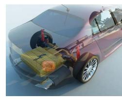
pure hydrogen gas stored directly on the vehicle and have the capability to refuel in as little as three minutes and can achieve a range of more than 300 miles on a single tank.
