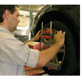
Tires are your car's critical connection to the road and can affect your ride, handling, traction and safety. Maintaining tire balance and wheel alignment reduces tire wear and improves handling and fuel economy.
