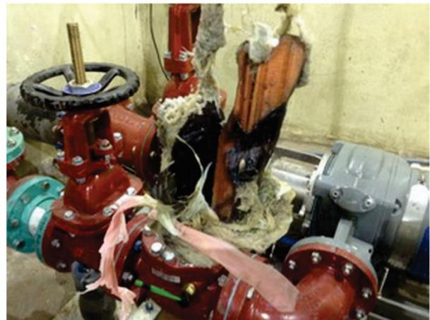
Pump failed due to clogging
