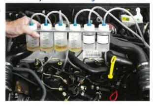
A fuel systems pressure is determined by its hydraulic integrity and injector backleakage is a key indicator of this. If backleak between the injectors is not uniform or excessive overall the system will fail to meet the demanded rail pressure. Backleakage should be checked using the Delphi Sealed Rail Kit YDT278 and if outside limits mentioned in the kit then the injectors should be serviced in accordance with Delphi standards or replaced.
