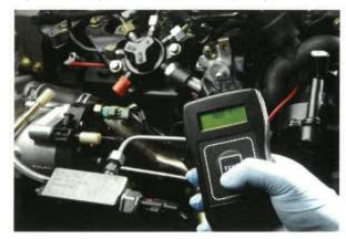
Using the Delphi Sealed Rail Diagnostic Kit YDT278 check the pressure and flow generated by the pump at cranking RPM. If the output is lower than specified in the kit instructions then the pump is worn and requires attention.
